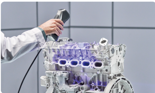
62 Line Full Field Structured Blue Light Scanning Capture Point Cloud Efficiently
